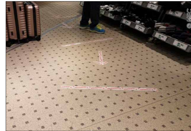
Separation of walking areas through the use of markings on floors and barrier tape
